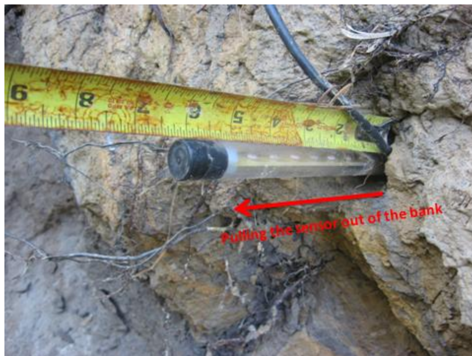
Figure 3.11: In-bank calibration of the PEEP.
