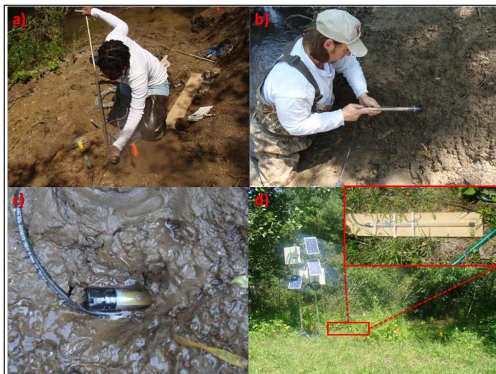
Figure 3.13: Installation procedure for the PEEPs.
