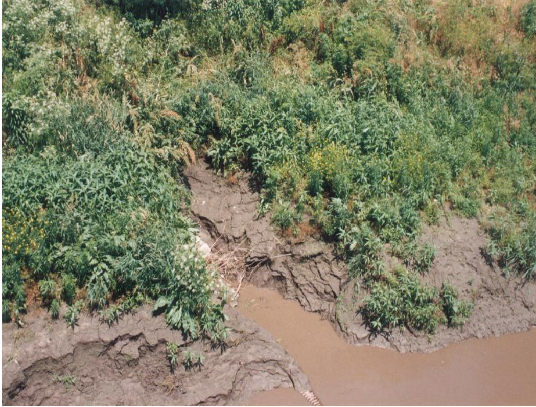
Figure 1.5: Pop-out failure in a cohesive lower bank (Midwestern US) (Papanicolaou et al., 2006)
